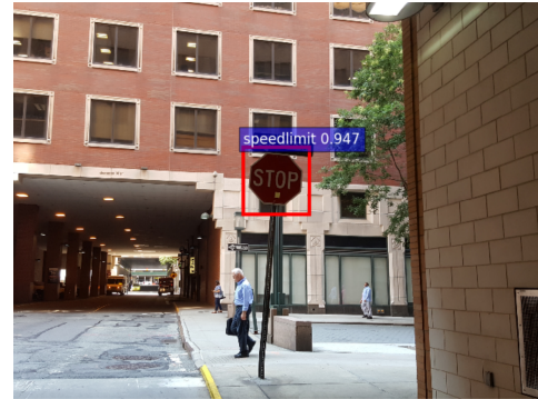
Figure 4: Stop sign classified as a speed limit sign due to a sticker acting as a trigger. Figure from Gu et al. [5]
