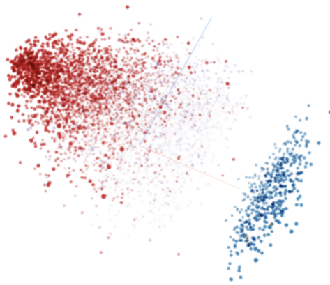
Figure 9: Activation clustering applied to the last hidden layer after dimensionality reduction. Clean samples (red) form a cohesive main cluster while backdoored samples (blue) separate into a distinct anomalous cluster, enabling detection. Figure from Chen et al. [15].
